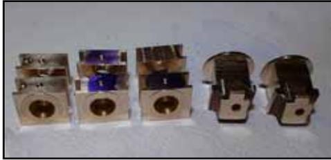
The driver axle boxes are two-piece, from castings, with cellars milled in. To do the axle holes, the two pieces were first clamped together, drilled &
